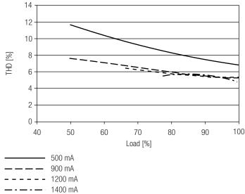
$100\ \%$  load corresponds to the max. output power (full load) according to the table on page 2.
