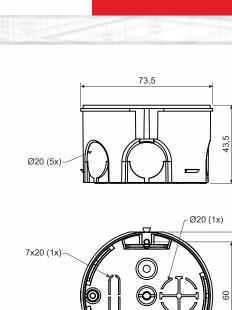
product description: designed for distribution system with voltage 400 V and with maximum current 16 A allows to install double-socket possibility to join into and continuous series with and spacing of 71 mm (up to 3 boxes) boxes can be joined with boxes KP 68/2, KP 68 and KPR 68 possibility to insert a terminal plate and screwless terminals
