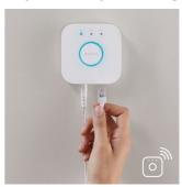
Connect your Philips Hue lights with the bridge to control your lights from your smart phone or tablet via the Philips Hue app.
