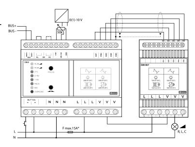
\* Potential L on device terminal needs to be protected by a protection element corresponding to load connected to the device.
