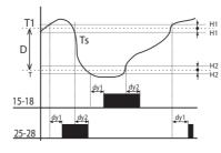
s - real (measured) temperature T1 - adjusted temperature
