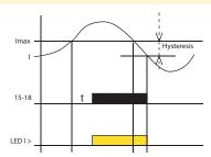
Monitoring relay PRI-52 serves for monitoring of current level in 1-phase AC circuits. Slight setting of release current level designates this relay for many various applications. Output relay is in normal status switched off. When set current level is overrun, relay get closed after preset delay. By return from error to normal status is used hysteresis.
