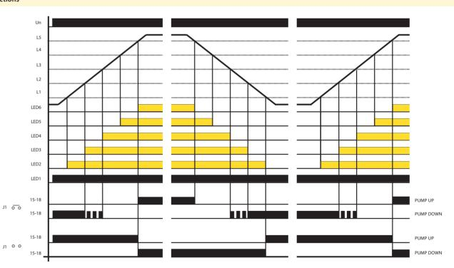
This device monitors level of a conuctive liquid in a tank by using six single probes or one 6-fold probe. In case you use a tank made of a conductive material, it is possible to use it as a common probe C.
